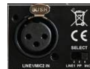
Phantom Power for Mic Input
