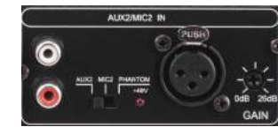
Phantom Power for Mic Input
