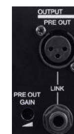
Line Output with Gain Control
