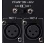
Mic 3 & Mic 4 with Phantom Power
